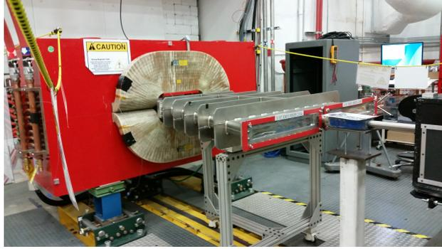
Figure 2.4: An image of the pair spectrometer in the hall. The beam travels from left to right across the image.
