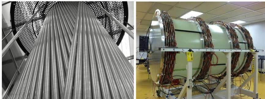
Figure 2.10: The drift chambers used in the GlueX experiment for charged particle tracking. On the left is the Central Drift Chamber (CDC) and on the right is the Forward Drift Chamber (FDC) [11].
