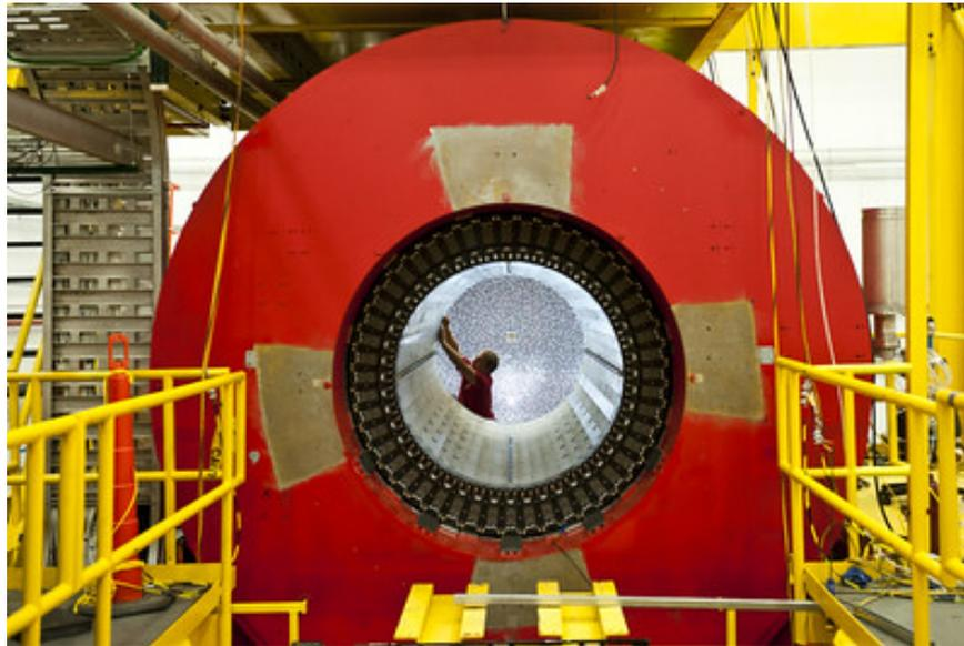
Figure 2.8: A picture of the superconducting solenoid being installed in Hall D. This is used to bend charged particles that enter to determine their momentum [10].
