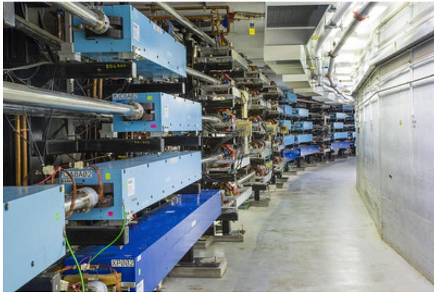
Figure 2.4: A picture of the RF linear accelerator portion of CEBAF. There are five beam pipes corresponding to the energy of the electrons. Lower energy electrons travel on the top beam pipes while higher energy electrons travel in the beam pipes closer to the ground [10].
