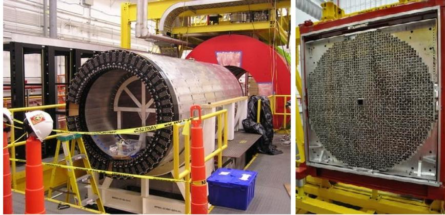
Figure 2.11: The calorimeters used in the GlueX experiment for neutral particle reconstruction and timing information. On the left is the Barrel Calorimeter (BCAL) and on the right is the Forward Calorimeter (FCAL) [11].
