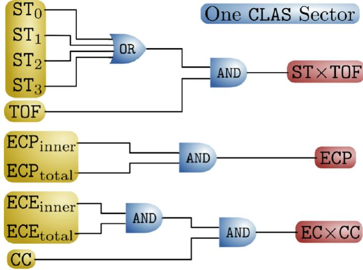
Figure 2.15: Illustrated are three distinct coincidence trigger criteria.  $ECP_{inner}$  and  $ECP_{total}$  represent a photon signal above threshold for the inner layer of the EC and entire EC respectively.  $ECP_{inner}$  and  $ECP_{total}$  represent an electron signal above threshold for the inner layer of the EC and entire EC respectively.  $ST_{0,1,2,3}$  are the four TDC signals for the start counter. Image source [42]
