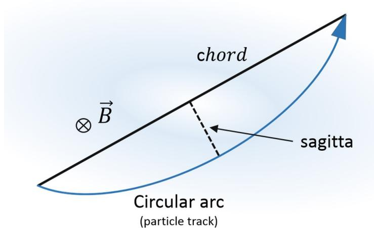
Figure 2.16: The path of a charged particle going through a magnetic field. When the radius of curvature is large when compared with the sagitta, the radius of curvature can be approximated by  $r \approx \frac{l^2}{2s}$ .
