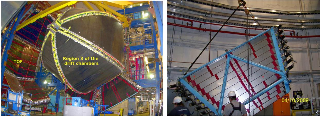
Figure 2.16: (Left) A photograph showing the time-of-flight detector as it was pulled away from the CLAS assembly during a maintenance period. Image source: [48]. Licensed under CC BY-SA 2.0. (Right) A picture of a section of a time-of-flight panel during installation. Note the photomultiplier tubes attached to the ends of the scintillating paddles. Image source: [58].
