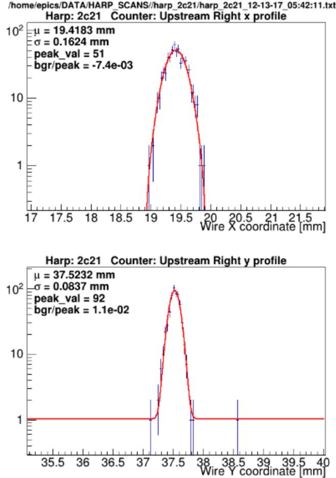
Figure 2.17: A typical harp scan to measure the electron beam profile. Shown are the  $x$  and  $y$  profiles of the electron beam just before hit the tagger. The orange lines is a Gaussian fit to the data. Image source [50].
