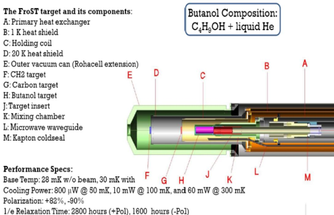
Figure 2.6: A cross section of the target area of FROST and its main components. Image source [38].
