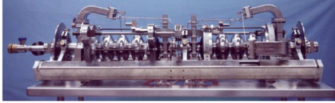
Figure 2.3: A pair of superconducting RF cavities with its support hardware and beam-pipe before transferred to the LINAC. Image source [41].
