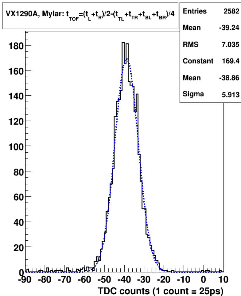
VX1290A<sub>TDC</sub>:  $\sigma(t_{TOF}) = \sim 100\text{ps}$  per plane including TDC resolution
