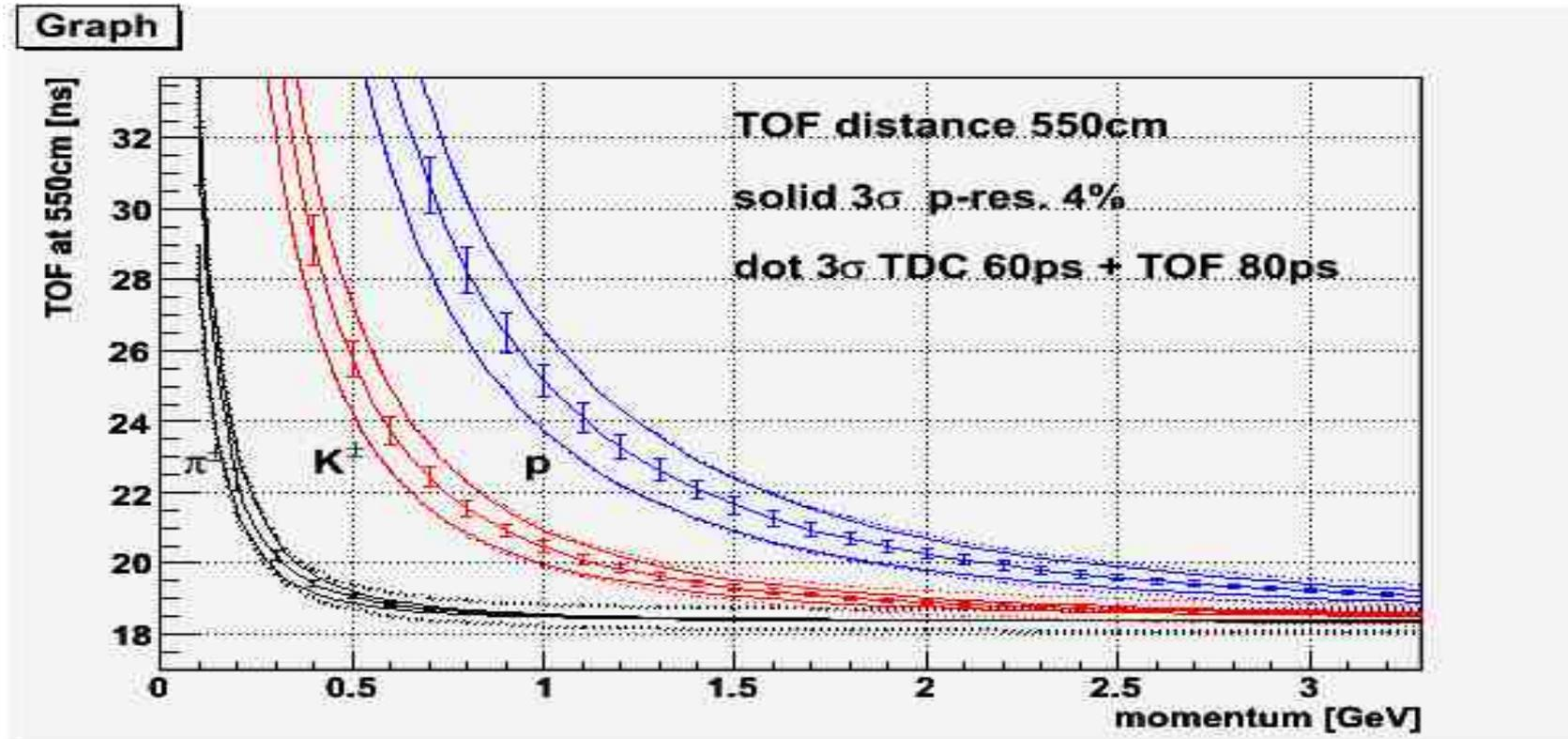
The above plot shows that the TOF system will be able to identify kaons with high efficiency and low contamination up to momenta of 2 GeV/c. Proton identification with very good efficiency and low contamination will be possible up to 3 GeV/c. This performance of PID at low momentum is nicely complementary to the momentum range of a RICH detector systems which can provide PID down to momenta of about 2 GeV/c.
