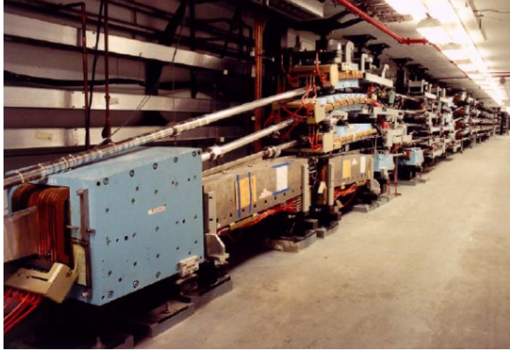
Figure 2.7: A picture inside the accelerator tunnel at Thomas Jefferson National Accelerator Facility; specifically the North Linac section of the accelerator which houses the magnets used to turn the electron beam. The blue box located in the lower left portion of the picture is the magnet responsible for splitting the electron beam into the monoenergetic beam bunches which will eventually continue into one of the five beam pipes in the picture. Farther down stream are several magnets used to steer the beam around the accelerator. Image source [8]
