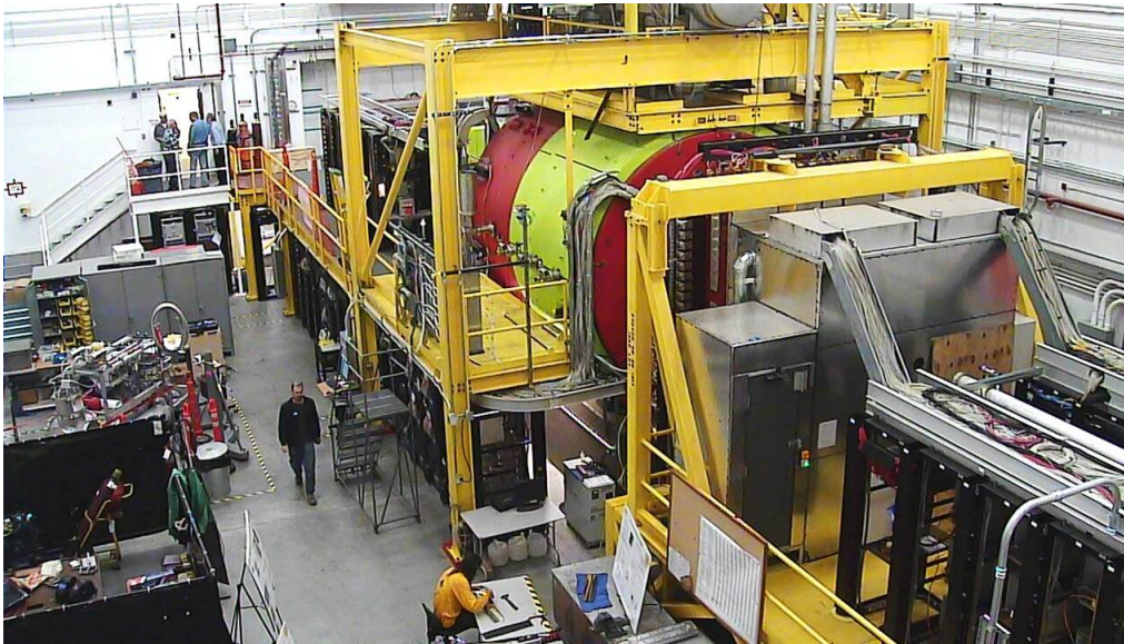
Figure 2.1: A picture taken from inside Hall D. From this angle, the photon beam would be coming towards the viewer, and eventually interact with the liquid hydrogen target located inside the apparatus. One can easily identify the shell of the superconducting barrel shaped solenoid as well as the back side of the forward calorimeter and some photomultiplier tubes attached to the time of flight detector. [8]
