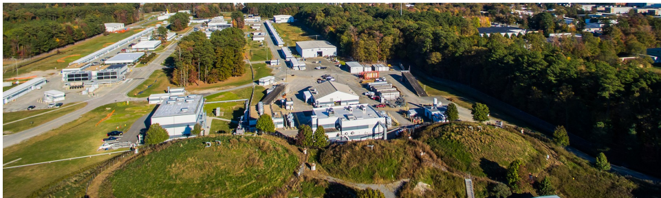
Figure 2.2: A picture taken of the Thomas Jefferson National Accelerator Facility (JLab) in Newport News, Virginia. In this picture, the electron beam from the Continuous Electron Beam Accelerator Facility (CEBAF) will travel in a clockwise motion. The two linear accelerator sections of the CEBAF are near the two parallel lab roads which run towards and away from the picture view. Three circular grass mounds can be observed in the lower part of this picture which represent the locations of Hall A, Hall B, and Hall C. Hall D is located diagonally across the CEBAF from those three halls and somewhat visible in this picture. [8]
