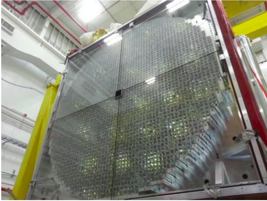
Figure 2.17: A picture of the forward calorimeter with no cover in front of it. One can clearly see the lead scintillators used to reconstruct photons in the forward direction. [4]
