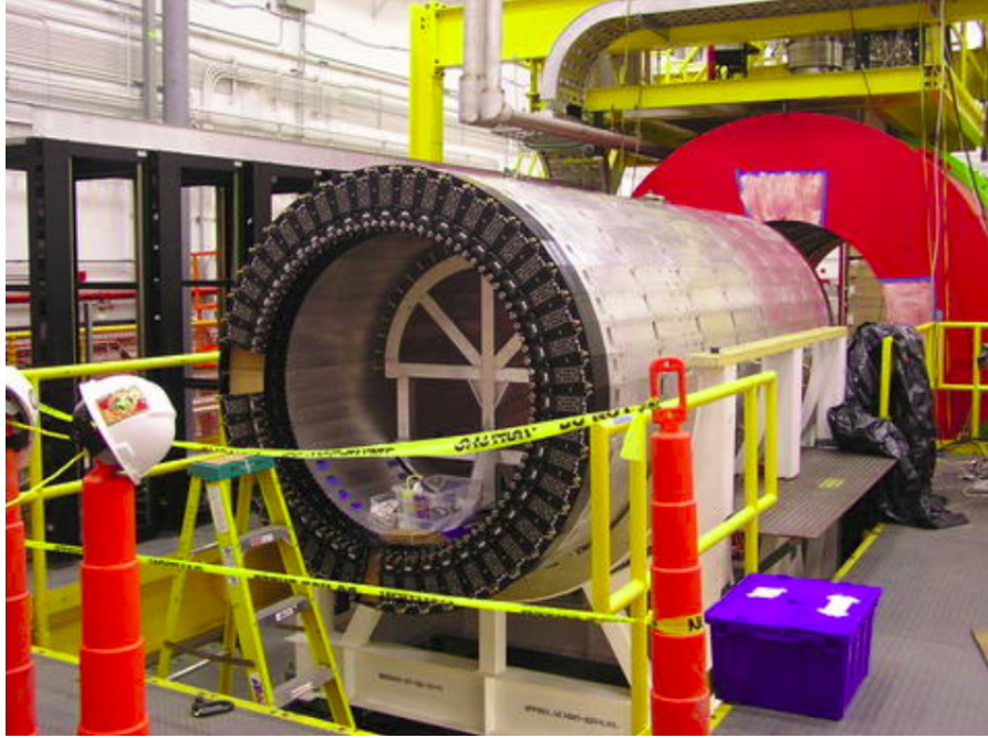
Figure 2.16: A picture of the barrel calorimeter before assembly into the superconducting solenoid. [4]
