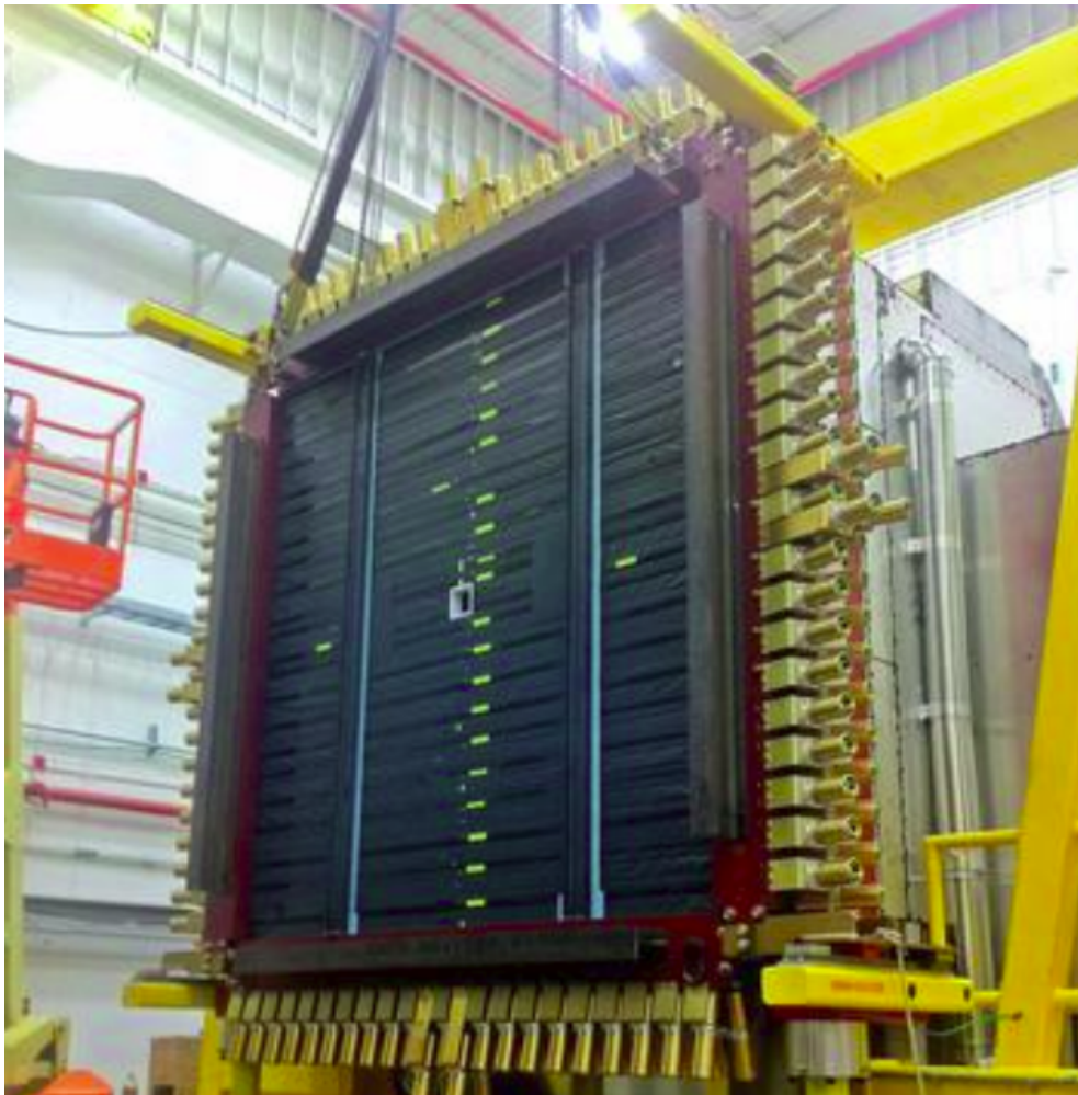
Figure 2.18: A picture of the time of flight after sucessful assembly inside Hall D. [4]
