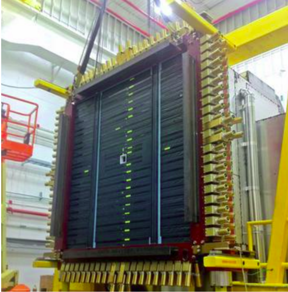
Figure 2.18: A picture of the time of flight after successful assembly inside Hall D. [4]
