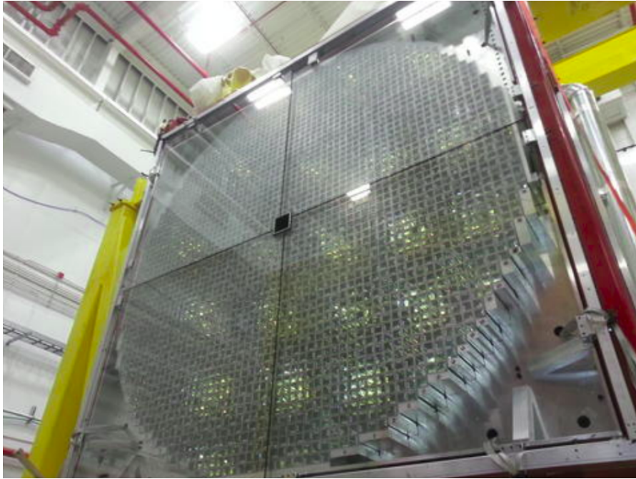
Figure 2.17: A picture of the forward calorimeter with no cover in front of it. One can clearly see the lead blocks used to reconstruct photons in the forward direction. [4]
