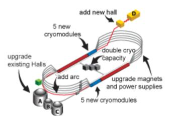
Figure 2.3: An illustration of the 12 GeV CEBAF upgrade at Jefferson Lab. This depiction shows where many of the aforementioned upgrades were physically placed within CEBAF and JLab. [19]
