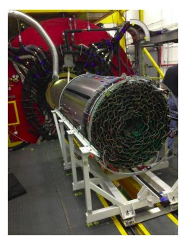
Figure 2.14: A picure taken of the central drift chamber before being installed into the GlueX spectrometer inside Hall D. [27]
