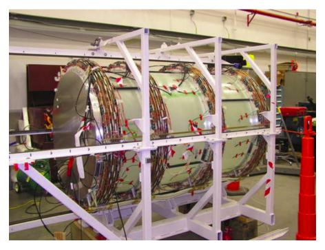
Figure 2.15: A picture taken of the forward drift chamber being surveyed on the floor of Hall D before installation. [27]
