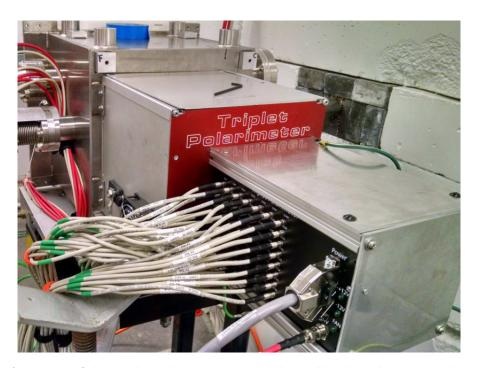
Figure 2.10: A picture of the triplet polarimeter inside the Hall D beamline. The photon beam will enter the triplet polarimeter from the upper left part of the picture and travel to the right. After interaction with the triplet polarimeter, an electron-positron pair will travel beyond the wall on the right portion of the photograph, where the pair spectrometer is located; as well as the GlueX spectrometer. [26]
