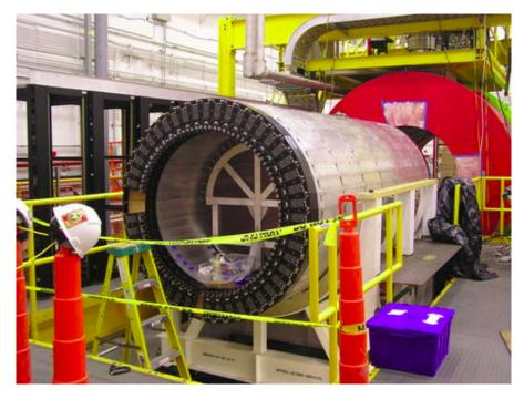
Figure 2.16: A picture of the barrel calorimeter before assembly into the superconducting solenoid. [27]
