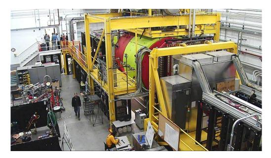
Figure 2.1: A picture taken from inside Hall D. From this angle, the photon beam would be coming towards the viewer, and eventually interact with the liquid hydrogen target located inside the apparatus. One can easily identify the shell of the superconducting barrel-shaped solenoid as well as the back side of the forward calorimeter and some photomultiplier tubes attached to the time of flight detector. [19]
