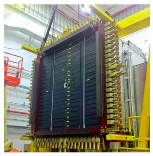
Figure 2.18: A picture of the time of flight after successful assembly inside Hall D. [27]
