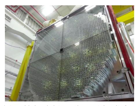
Figure 2.17: A picture of the forward calorimeter with no cover in front of it. One can clearly see the lead blocks used to reconstruct photons in the forward direction. [27]
