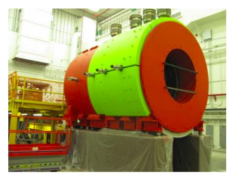
Figure 2.13: A picure taken of the solenoid located inside Hall D. [32]
