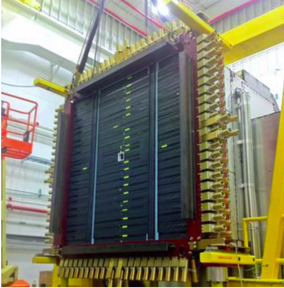
Figure 2.18: A picture of the time of flight after sucessful assembly inside Hall D. [28]
