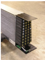
Barrel CALorimeter (BCAL): 48 4-m long modules
