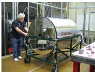
CDC: 28-layer straw-tube chamber
