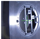
Goniometer: 20 \mu\text{m} diamond
