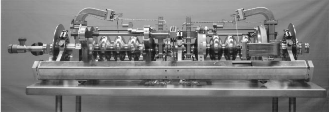
Figure 2.1: A photograph of a typical cavity used at CEBAF, made up of two superconducting niobium klystrons. A positive potential is applied across each cavity in turn as an electron bunch passes through, providing a constant acceleration gradient. This alternating of potentials down each linac amounts to a standing electromagnetic wave at radio frequencies within the cavity; the superconducting walls of the cavity ensure that almost all of the energy of the standing EM wave goes into the electrons passing through. (Image source: [54]).
