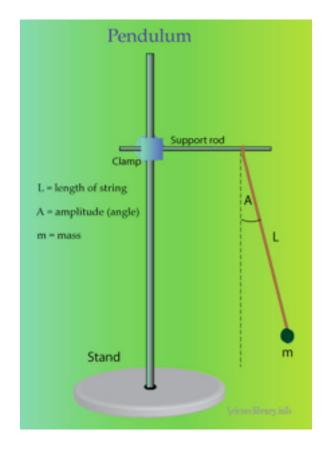
Determine how the amplitude of the motion, the mass of the object, and the length of the string affect the period of the motion.
