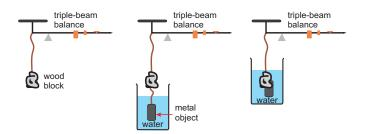
If we do this, we can compute the specific gravity of wood by using the relationship
