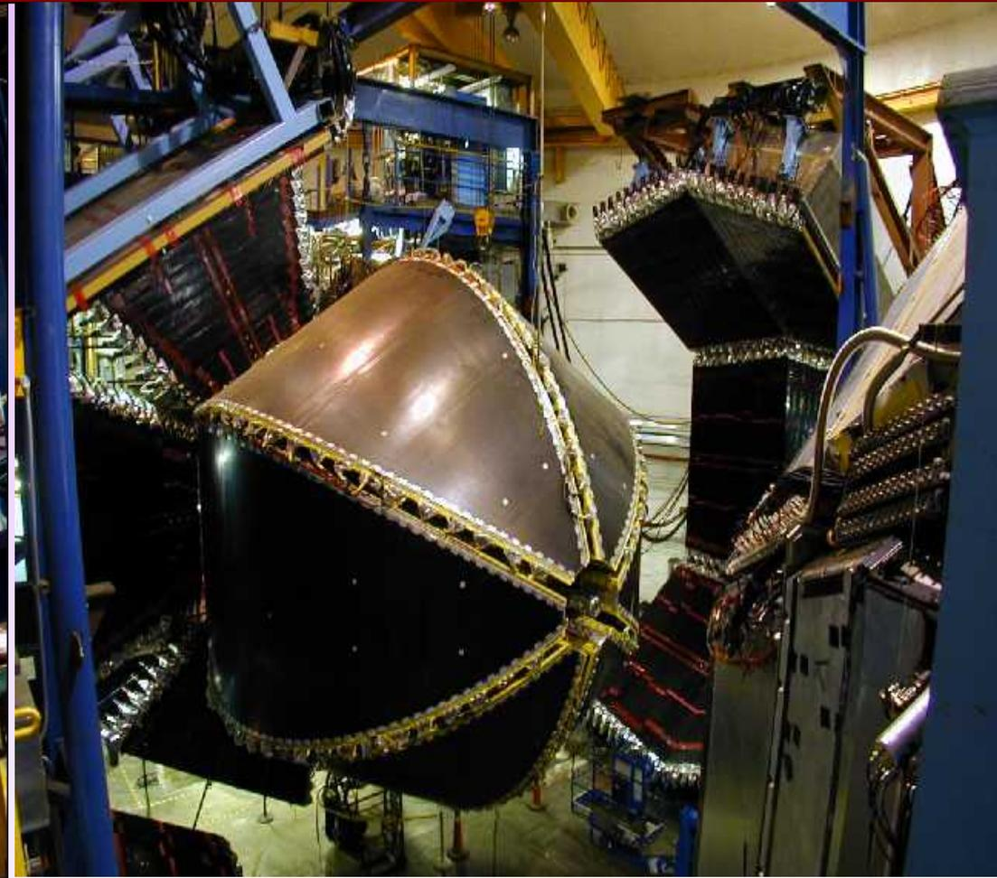
◆ Skeletal superconducting Toroidal Magnets for CLAS.
