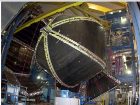
CLAS detector- charged particles detection, almost  $4\pi$  coverage
