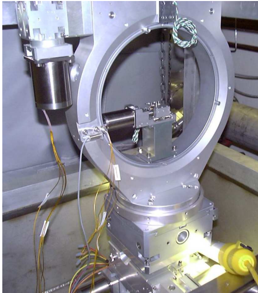
Figure 2.6: (Left) The goniometer used in Hall B to adjust the coherent edge position and orient the polarization plane of the photon beam parallel or perpendicular to the floor. (Right) A diagram of a target ladder containing various radiators. It was placed at the center of the goniometer. The required radiator could be moved into position when needed.
