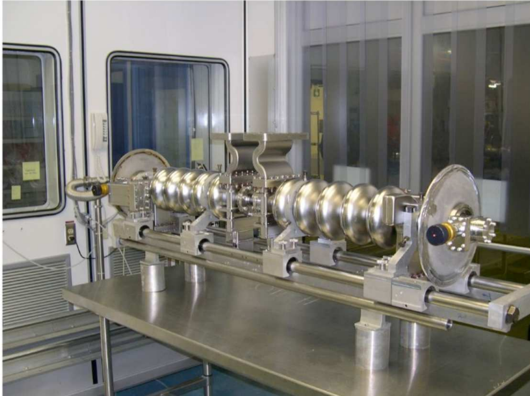
Figure 2.2: A picture of a cryomodule consisting of eight RF cavities. Image source: [45].
