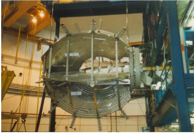
Figure 2.15: (Left) A picture of the Torus magnet during installation in Hall B. The kidney-shaped superconducting coils are shown in the picture. (Right) A map of the magnetic field vectors on a plane which is perpendicular to the beam line and centered on the target. The length of each line segment is proportional to the magnetic field strength at that point. The field vectors primarily point in the \phi direction. The gray bars are the six coils in the cross section. Image sources: [54], [55].
