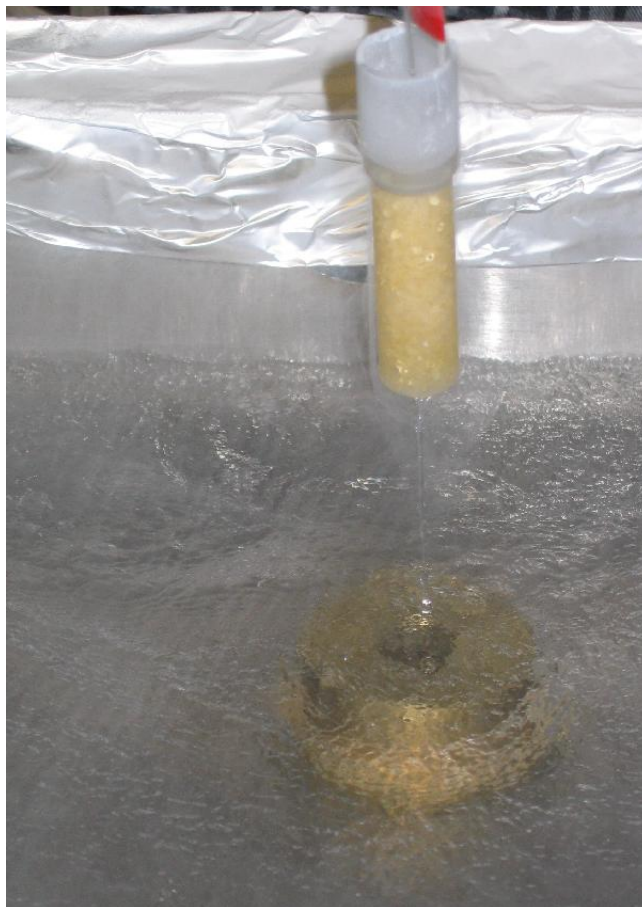
Figure 3.7: The target cup coming out of the liquid nitrogen submersion filled with butanol beads and ready to be placed in the target [7].
