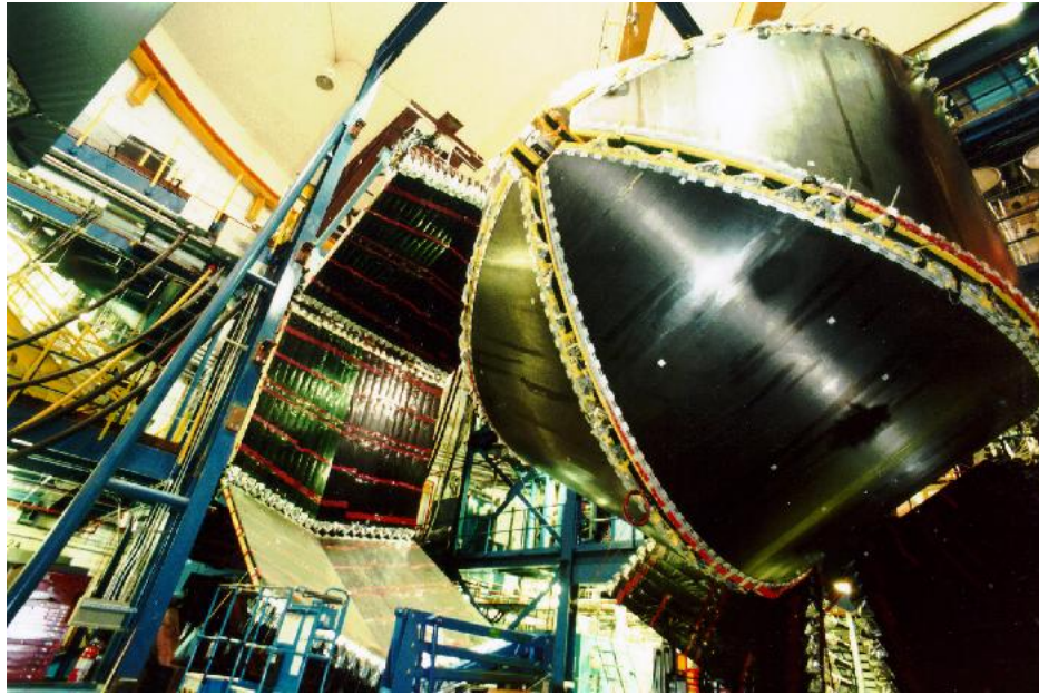
Figure 3.11: The CEBAF Large Acceptance Spectrometer. The time-of-flight clamshells are exposed in this image, showing the drift chambers surrounding the target enclosure [8].
