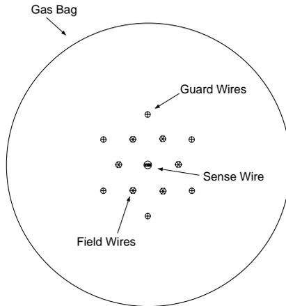
Figure 1: Schematic representation of one of the individual drift cells of the prototype. Figure is drawn roughly to scale.
