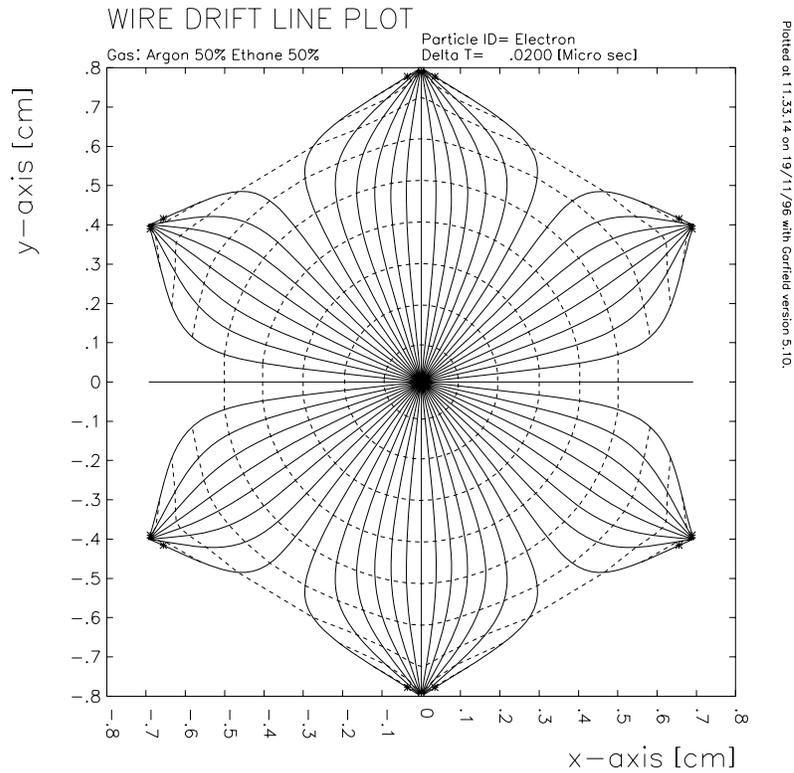
Figure 3: Results of a GARFIELD field line calculation of a single prototype drift cell in a 50-50 argon/Ethane environment with  $V_{field} = -2400\text{ V}$ ,  $V_{guard} = -1200\text{ V}$ , and  $V_{sense} = 0\text{ V}$ .
