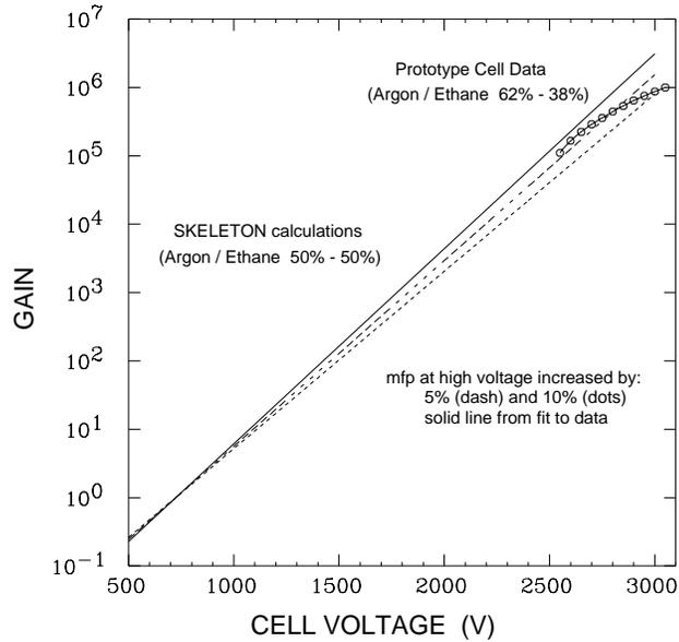
Figure 11: Measured gain averaged over the six individual drift cells plotted as a function of the magnitude of the field voltage for argon/ethane (62% - 38% molar) compared with the results of the SKELETON gas gain calculation assuming an argon/ethane (50% -50%) mixture. The mean free path at high voltages was varied in the different calculations by 5% and 10% relative to the fit value.
