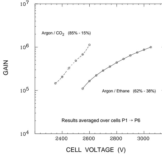
Figure 8: Measured gain averaged over the six individual drift cells plotted as a function of the magnitude of the field voltage. Measurements are shown for both argon/ethane (62% - 38% molar) and argon/CO<sub>2</sub> (85% - 15% molar).
