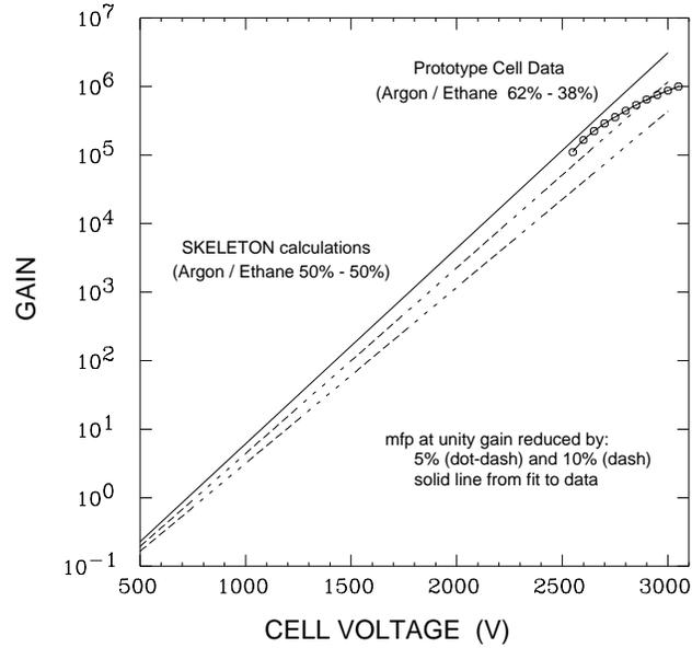
Figure 10: Measured gain averaged over the six individual drift cells plotted as a function of the magnitude of the field voltage for argon/ethane (62% - 38% molar) compared with the results of the SKELETON gas gain calculation assuming an argon/ethane (50% -50%) mixture. The mean free path at unity gain was varied in the different calculations by -5% and -10% relative to the fit value.
