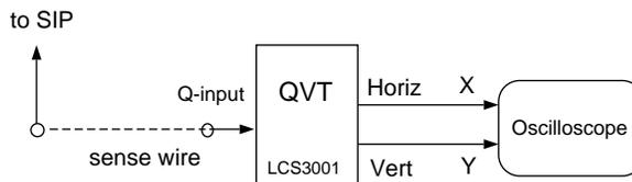
Figure 7: Electronics configuration for the drift cell gain measurements.
