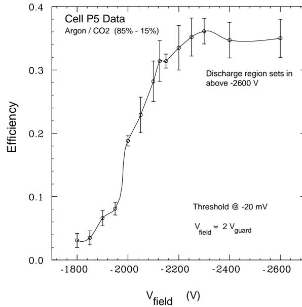
Figure 5: Cell P5 efficiency measured as a function of the field voltage in an argon/ $\text{CO}_2$  (85% - 15% molar) environment at a threshold of -20 mV.
