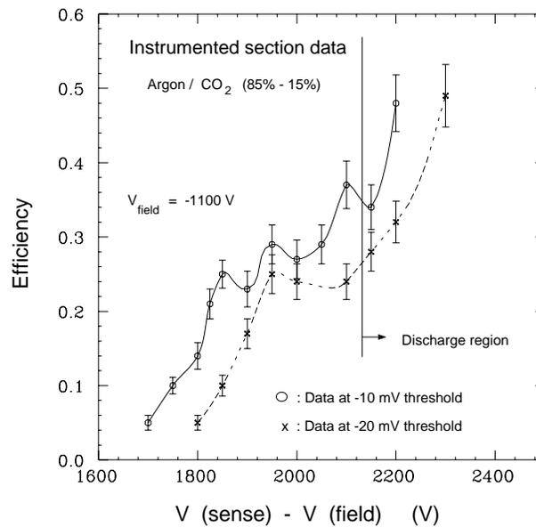
Figure 6: Instrumented section efficiency measured as a function of the difference between the sense and field voltages in an argon/ $\text{CO}_2$  environment at thresholds of -10 mV and -20 mV.
