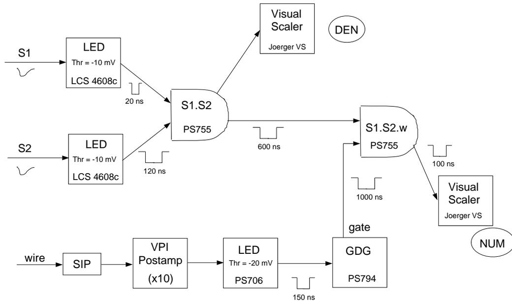
Figure 4: The top half of this figure shows the detector layout for the efficiency measurement of drift cell P5. The bottom half of this figure shows the electronics scheme for the measurement.
