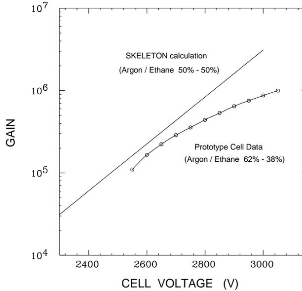
Figure 9: Measured gain averaged over the six individual drift cells plotted as a function of the magnitude of the field voltage for argon/ethane (62% - 38% molar) compared with the results of the SKELETON gas gain calculation assuming an argon/ethane mixture (50% -50%).
