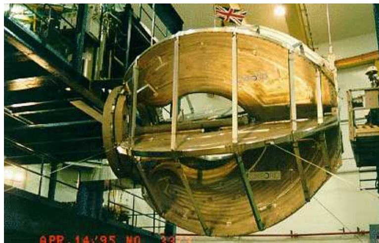
Figure 2.12: The coils of the CLAS toroidal magnet prior to installation of the rest of the detector subsystems. Image Source: [33].
