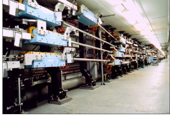
(b) North Linac Beam Recombiner. The blue boxes on the beam-lines are powerful electromagnets required to join the mono-energetic components of the electron beams into a single multi-energy electron beam.
