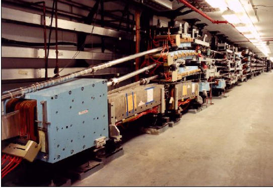
(a) North Linac Beam Spreader. The blue boxes on the beam-lines are powerful electromagnets required to split a multi-energy beam into its mono-energetic components.
