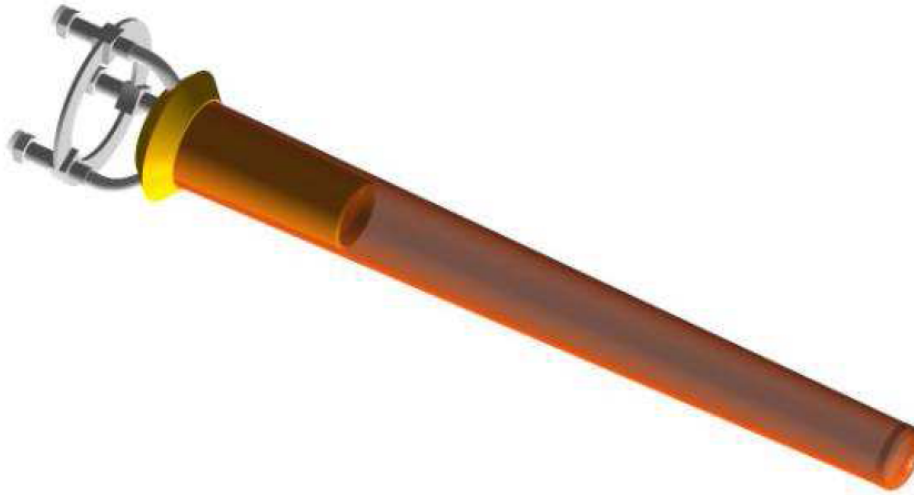
Figure 2.13: 40 cm long kapton target used during the g12 run, placed 90 cm upstream of the CLAS center, filled with liquid hydrogen ( LH_2 ). Image source [32].
