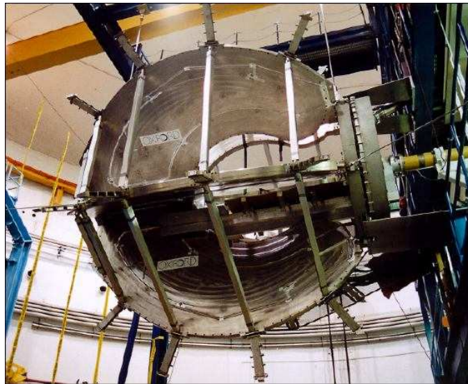
Figure 4.9: Photograph of the torus magnet cryostats, showing one of the two support rings on which they are mounted and the carbon-fibre support rods between neighbouring cryostats (Jefferson Lab Hall B archive).
