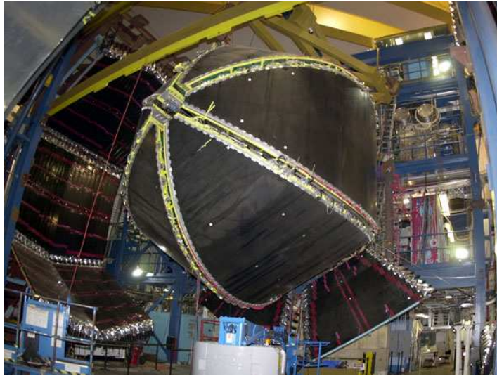
Figure 4.12: Photograph of CLAS opened up, showing, from the upstream end, the sphere formed by the six sectors of the drift chambers. At the left edge of the photograph and in the bottom right corner (behind the drift chambers), the wrapped scintillator paddles of the time-of-flight system can be seen (Jefferson Lab Hall B archive).
