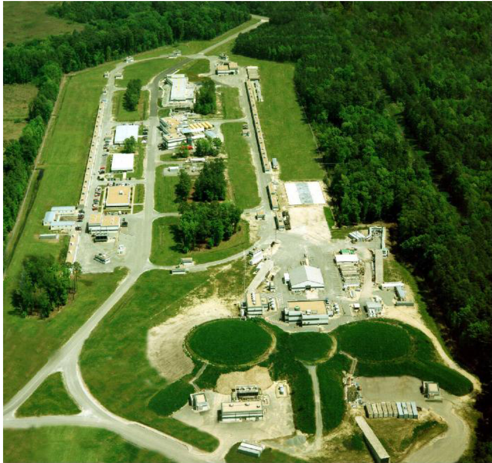
Figure 1: The CEBAF accelerator as viewed from the air. The accelerator is beneath the roads tracing out a racetrack shape, and Halls C, B, and A (left to right) are visible at the bottom.
